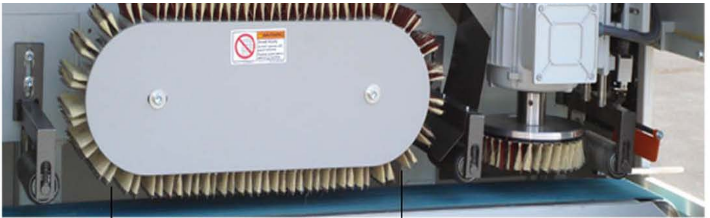
The sanding area of the belt is approximately five times larger compared to a standard brush roller
