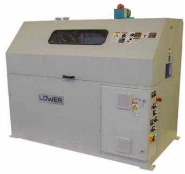
The LÖWER MultiMaster LZ 3DB-150 is a multi-sided sander designed for finish sanding and denibbing of all types profiles and mouldings. Sanding strip units process all surfaces and profiles simultaneously from above, left and right. The MultiMaster LZ 3DB is available in a working width of 150mm (6").
