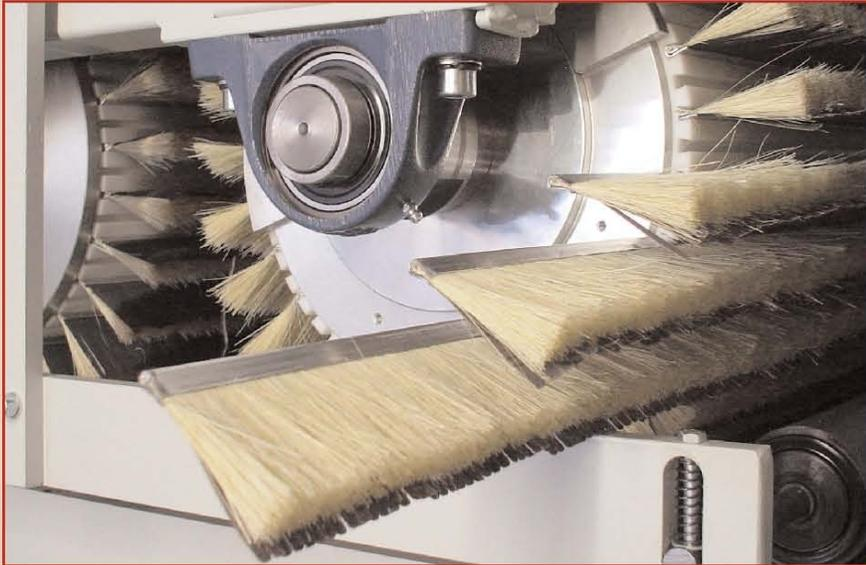
The Smart-Flex system is very economic as only the sanding strips need to be replaced. Thanks to the split end cap (optional extra), the sanding strips can be changed in minutes without removing the core from the machine - this means even shorter machine down times.
