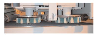
Additional hold down roller between discs for better transport of small work pieces even without vacuum
